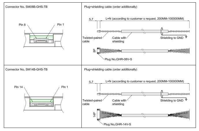
8.2 Radial Cable Schematic
